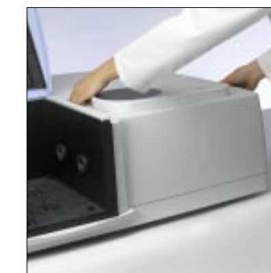
Taking out the transmission module and replacing it with the Universal Reflectance Accessory (URA)
