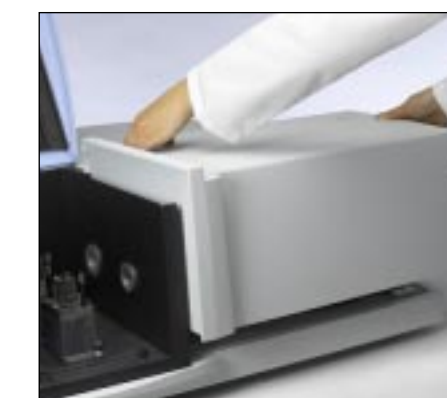
Taking out the transmission module and replacing it with the Universal Reflectance Accessory (URA)
