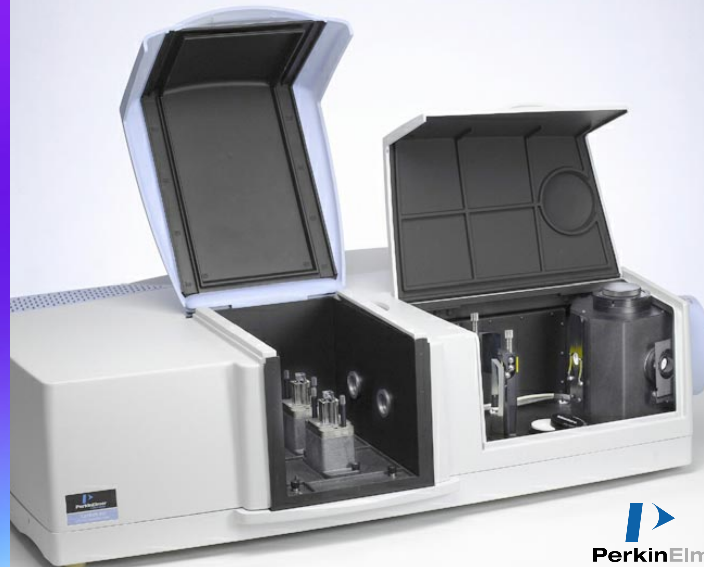
The dual sampling areas on the LAMBDA™ 950, 850 and 650.
